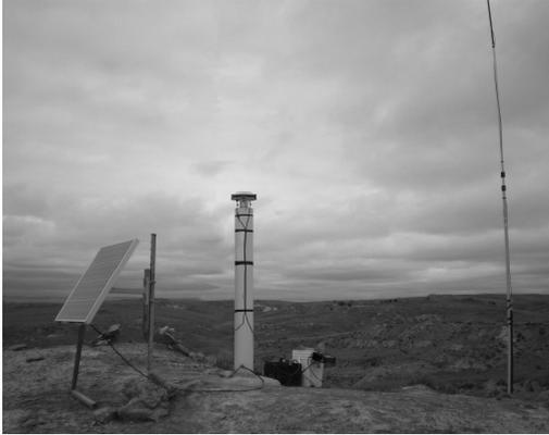
Figure 2. GPS base with associated equipment. Blue radio is near battery power source on right. Solar panel on left used to maintain charge. Tall mast on far right is radio antenna.
